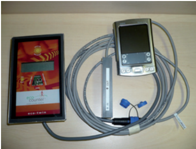
Figure 3 – Monitoring equipment (pyroelectric sensor, data logger and palmtop)
